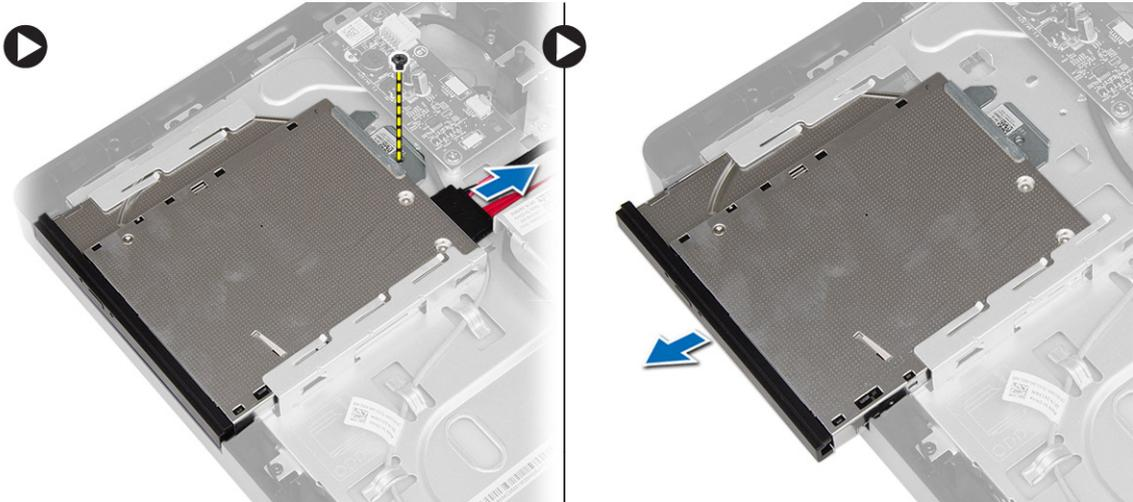
4. Remove the screws that secure the bracket to the optical disk drive and remove it from the optical drive.
