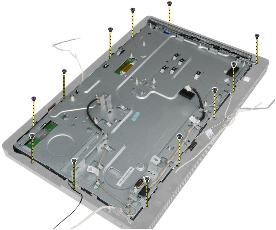
5. Release the display bracket from its tab on the chassis and remove it from the computer.
