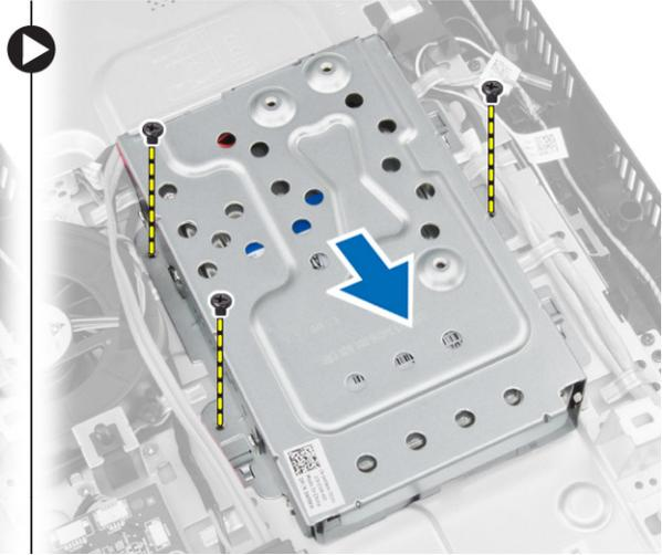
4. Turn and place the hard drive on the hard-drive bracket to access the hard-drive cable. Disconnect the hard-drive cable from the hard drive.
