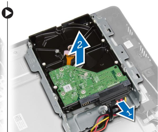
5. Remove the screws that secure the hard-drive bracket to the hard drive and remove the hard drive from the hard-drive bracket.
