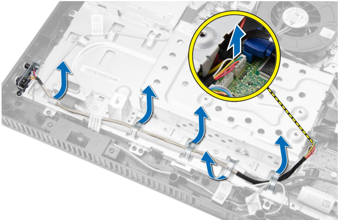
4. Remove the screw that secures the power switch to the computer. Release and remove the power switch from the computer.
