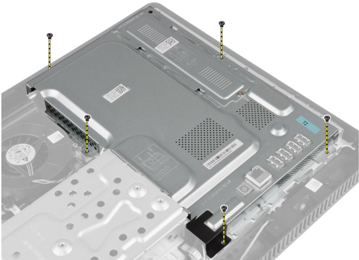
4. Lift the system board cover up to remove it from the computer.
