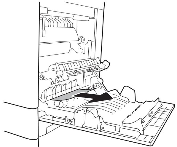
3. If paper is visible entering the bottom of the fuser, gently pull downward to remove it.
