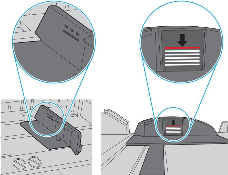
**Figure 6-7** Tab for the paper stack
