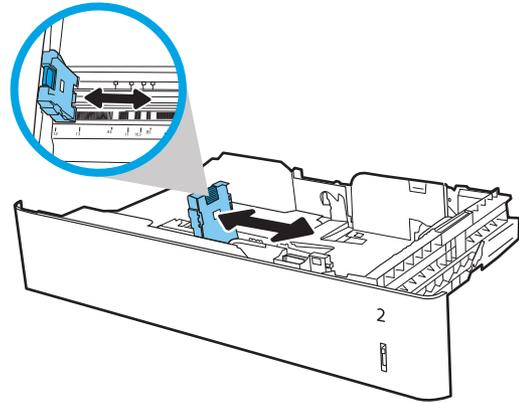
4. Load paper into the tray. Check the paper to verify the guides lightly touch the stack, but do not bend it. For information about how to orient the paper, see [Table 2-2 Tray 2 and the 550-sheet trays paper orientation on page 26](#).
