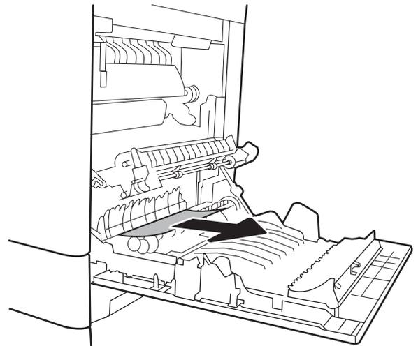
7. If paper is visible entering the bottom of the fuser, gently pull downward to remove it.
