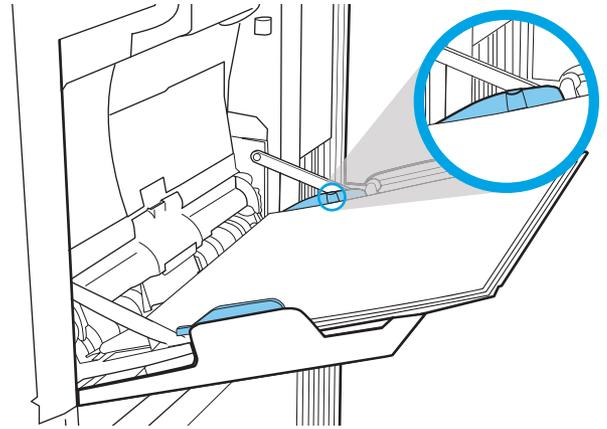
4. Using the blue adjustment latch, adjust the side guides so that they lightly touch the paper stack, but do not bend it.
