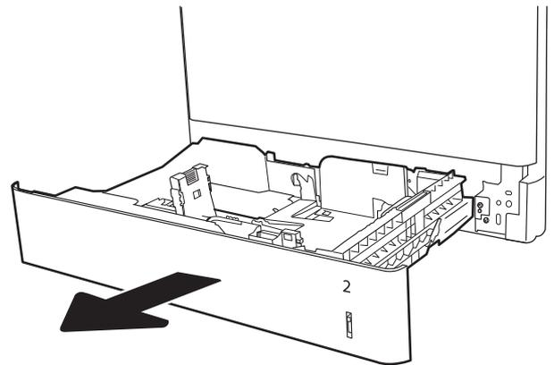
2. Before loading paper, adjust the paper-width guides by squeezing the blue adjustment latches and sliding the guides to the size of the paper being used.
