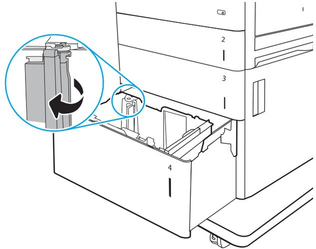
4. Load paper into the tray. Check the paper to verify the guides lightly touch the stack, but do not bend it. For information about how to orient the paper, see [Table 2-3 High-capacity input tray paper orientation on page 31](#).
