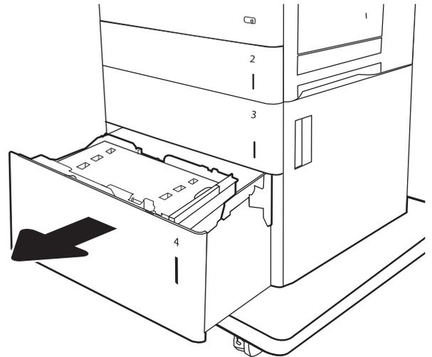
2. Before loading paper, adjust the paper-width guide by squeezing the blue adjustment latch and sliding it to the size of the paper being used.
