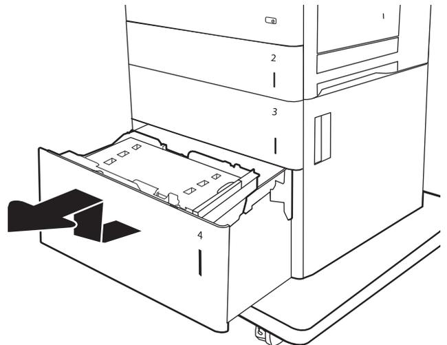
6. If jammed paper is in the feed area, pull it down to remove it. First pull the paper to the left to release it, and then pull it forward to remove it.
