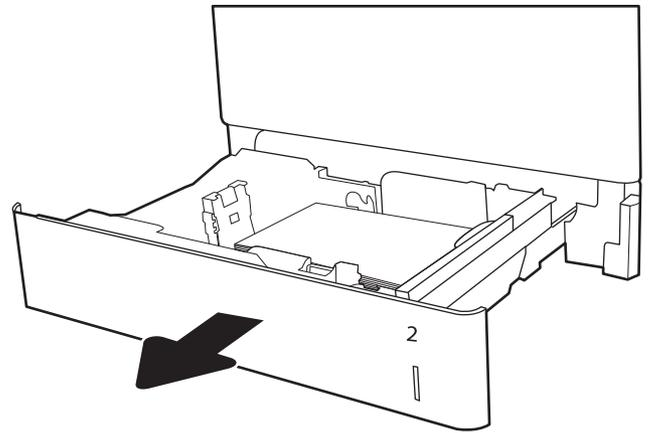
2. Remove any jammed or damaged sheets of paper. Verify that the tray is not overfilled and that the paper guides are adjusted correctly.
