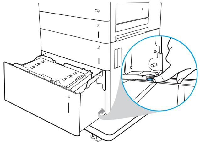
5. Lift the tray up and then pull it straight out to remove it.
