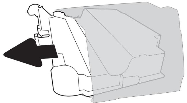
6. Install the new unit into the printer. Make sure the toner-collection unit is firmly in place.
