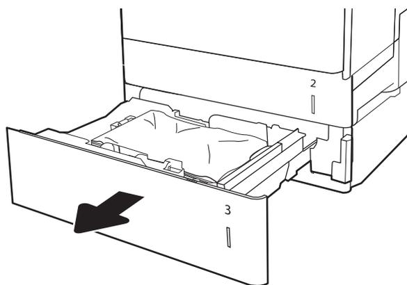
2. Remove any jammed or damaged sheets of paper. Verify that the tray is not overfilled and that the paper guides are adjusted correctly.
