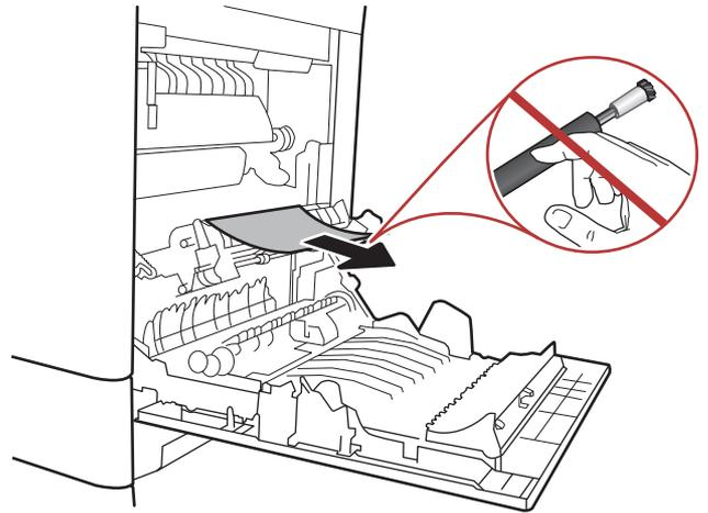
8. If paper is jammed as it enters the output bin, gently pull the paper out to remove it.
