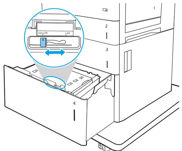
3. Rotate the paper-stop lever to the correct position for the paper being used.
