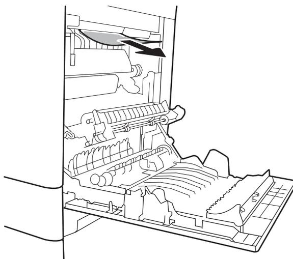
12. Paper could be jammed inside the fuser where it would not be visible. Grasp the fuser handles, lift up slightly, and then pull straight out to remove the fuser.
