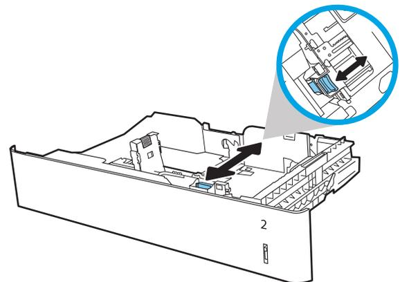
3. Adjust the paper-length guide by squeezing the adjustment latch and sliding the guide to the size of the paper being used.
