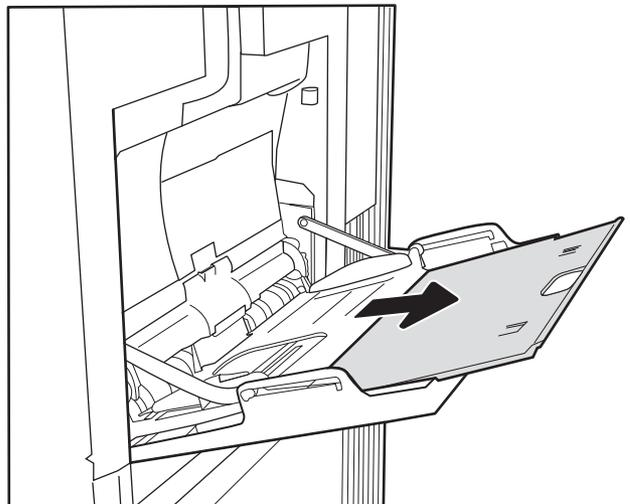
3. Use the blue adjustment latch to spread the paper guides to the correct size, and then load paper in the tray. For information about how to orient the paper, see [Table 2-1 Tray 1 paper orientation on page 20](#).
