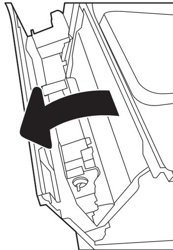
4. Grasp the top of the toner-collection unit and remove it from the printer.
