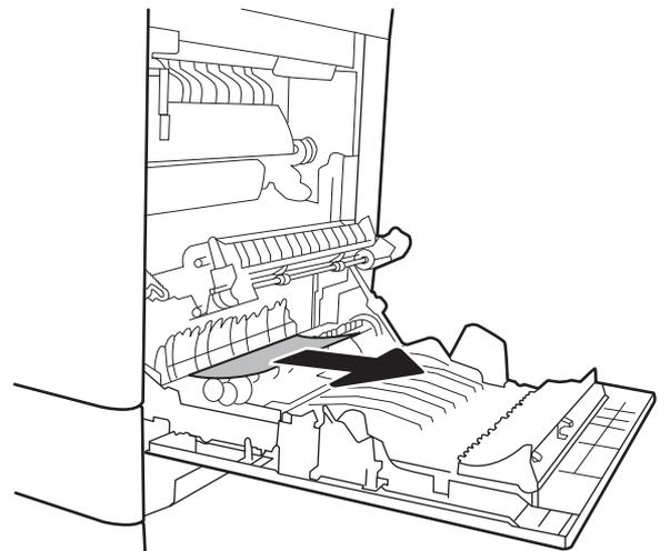
10. If paper is visible entering the bottom of the fuser, gently pull downward to remove it.
