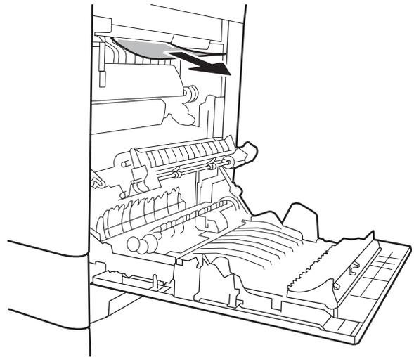
5. Paper could be jammed inside the fuser where it would not be visible. Grasp the fuser handles, lift up slightly, and then pull straight out to remove the fuser.
