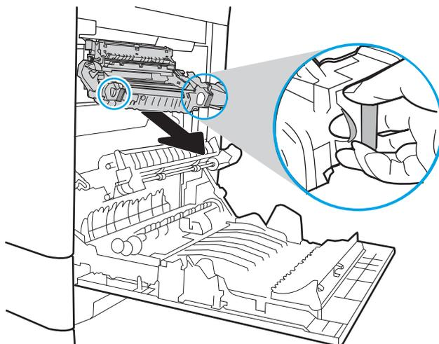
13. Open the jam-access door on the fuser. If paper is jammed inside the fuser, gently pull it straight up to remove it. If the paper tears, remove all paper fragments.
