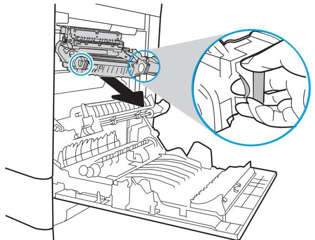
10. Open the jam-access door on the fuser. If paper is jammed inside the fuser, gently pull it straight up to remove it. If the paper tears, remove all paper fragments.
