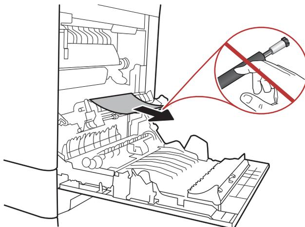
11. If paper is jammed as it enters the output bin, gently pull the paper downward to remove it.
