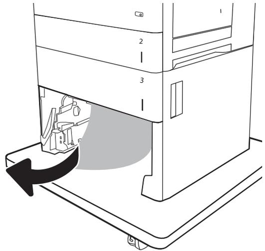
7. Install the tray, and then load full reams of paper into the tray. Verify that the tray is not overfilled and that the paper guides are adjusted correctly.
