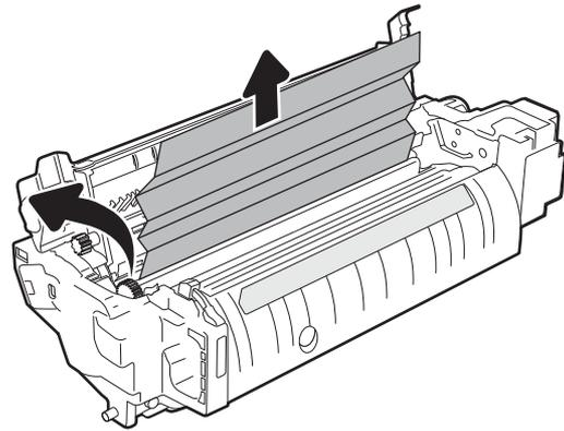
7. Close the jam-access door on the fuser, and push the fuser completely into the printer until it clicks into place.
