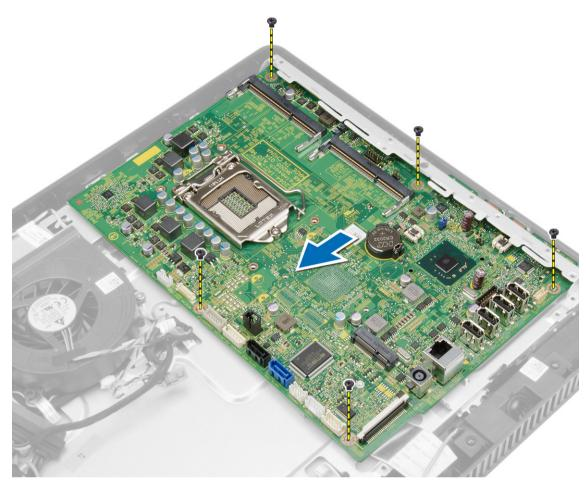
5. Lift the system board from one side to remove it from the computer.
