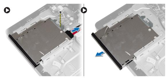
4. Remove the screws that secure the bracket to the optical disk drive and remove it from the optical drive.
