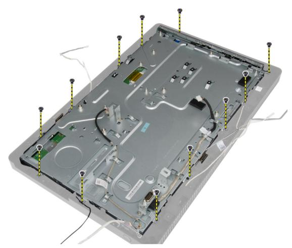
5. Release the display bracket from its tab on the chassis and remove it from the computer.
