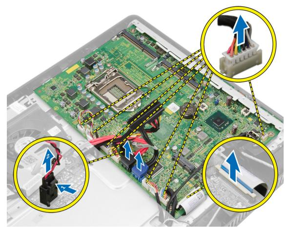
4. Remove the screws that secure the system board to the chassis of the computer and slide the system board to release it from the chassis.
