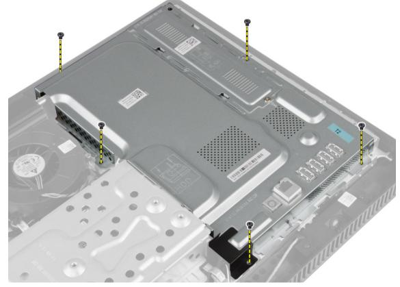
4. Lift the system board cover up to remove it from the computer.
