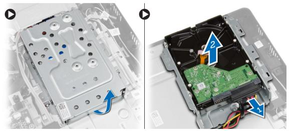
5. Remove the screws that secure the hard-drive bracket to the hard drive and remove the hard drive from the hard-drive bracket.
