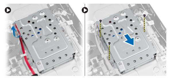
4. Turn and place the hard drive on the hard-drive bracket to access the hard-drive cable. Disconnect the hard-drive cable from the hard drive.
