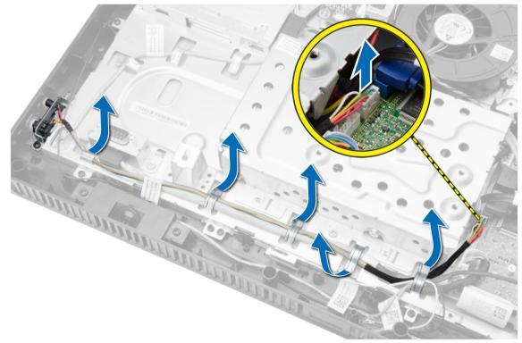
4. Remove the screw that secures the power switch to the computer. Release and remove the power switch from the computer.
