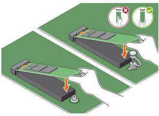
d If the system is shipped with screw tighten that secures the M.2 Intel optane memory module on the computer. If the system is shipped with self locking spacer press to lock the M.2 Intel optane to secure on the computer.
