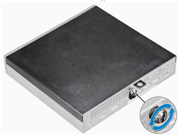
b Slide and lift the cover to remove from the computer.
