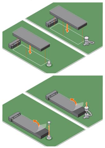
$\ensuremath{\text{c}}$  Place the M.2 Intel optane memory module into the slot on the thermal pad.
