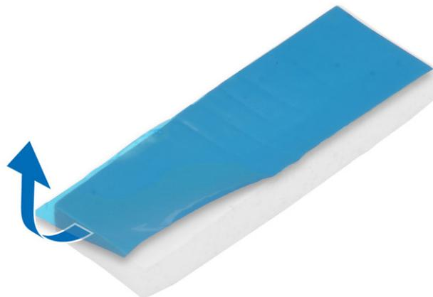
4. Place the rubber on the system board [1] and peel the adhesive tape (pink) from the rubber [2].
