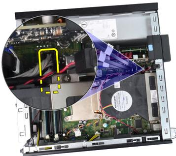
7. Remove the single screw that secures the I/O panel to the chassis.
