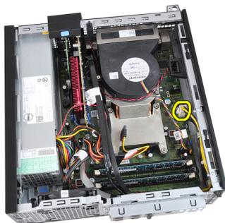
7. Unthread the 4-pin power cable from the chassis clips.
