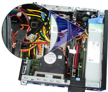
7. Press the speaker securing tab, and slide the speaker towards the right of the computer to release it.
