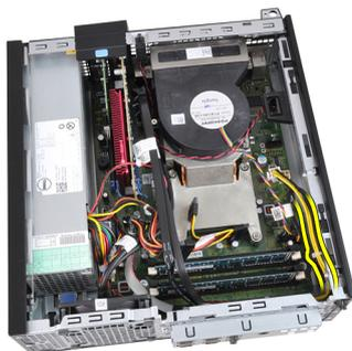
8. Disconnect the 24-pin power cable from the system board.
