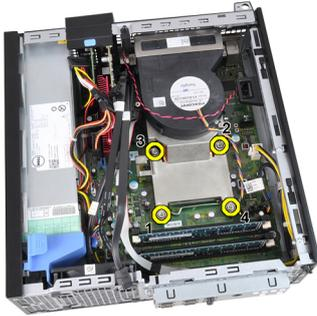
8. Lift the heat sink assembly upwards, and remove it from the computer. Lay the assembly with the fan facing downwards, and with the thermal grease facing upwards.
