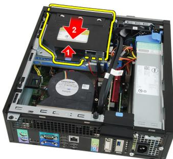
5. Remove the optical drive from the bracket.
