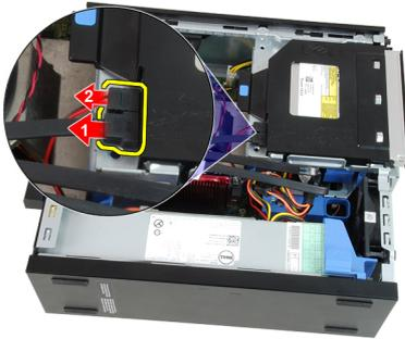
5. Slide the drive-cage handle toward the back of the computer into the unlocked position.
