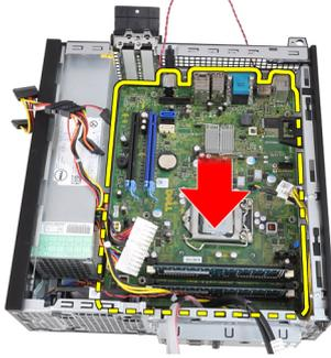
13. Remove the system board from the chassis.
