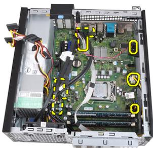
9. Lift and release the expansion-card latch, to gain access to the screws securing the system board.
