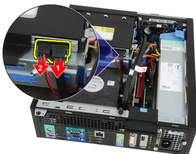
4. Lift the blue tab and slide the optical drive inwards to remove it from the computer.
