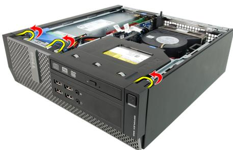
4. Rotate the bezel away from the computer to release the hooks on the opposite edge of the bezel from the chassis.
