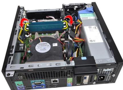
6. Lift the memory modules out of the connectors on the system board.
