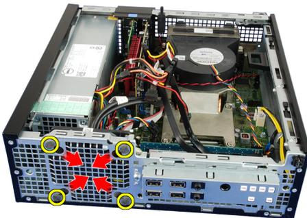
8. Lift and remove the system fan from the computer.
