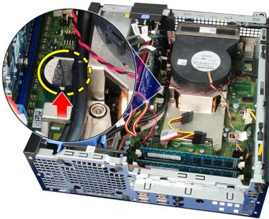
5. Lift the coin-cell battery out of the computer.
