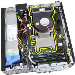
9. Press the release lever down and then move it outward to release it from the retention hook that secures it.
