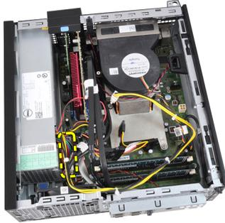
9. Remove the screws that secure the power supply, from the back of the computer.
