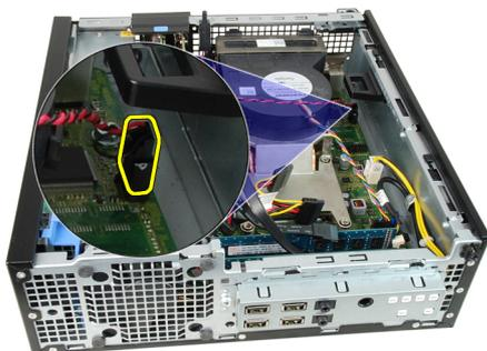
4. Slide the intrusion switch inwards and remove it from the system board.
