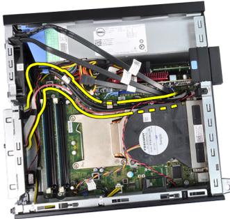
6. Disconnect the I/O panel or the FlyWire cable from the system board.
