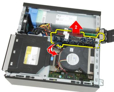
6. Pull the release lever away from the PCIe x4 card (if any) to release the securing tab from the dent in the card. Then, ease the card up and out of its connector and remove it from the computer.
