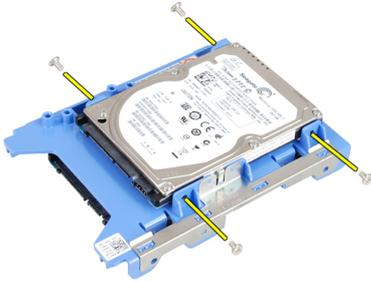
7. Release the screws that secure the 2.5 inch hard drive to the underside of the hard-drive bracket.
