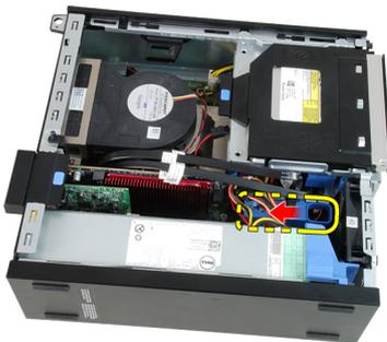
6. Rotate the drive cage upward using the handle and lift the drive cage free off the chassis.
