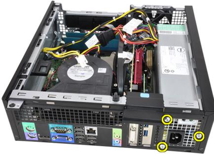
10. Push in on the blue release tab beside the power supply, and slide the power supply towards the front of the computer.
