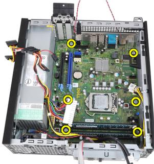
**11.** Remove the 7-mm hex screw that secures the system board to the chassis.
