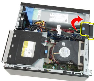
5. Pull the release lever away from the PCIe x16 card until you release the securing tab from the dent in the card. Then, ease the card up and out of its connector and remove it from the computer.
