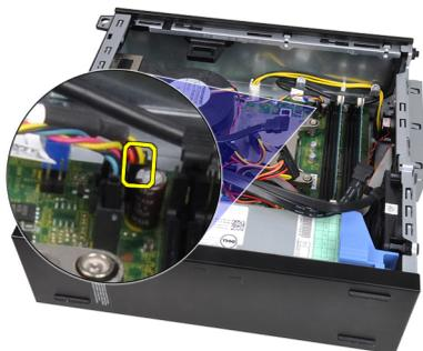
6. Unthread the power-switch cable from the chassis clip.
