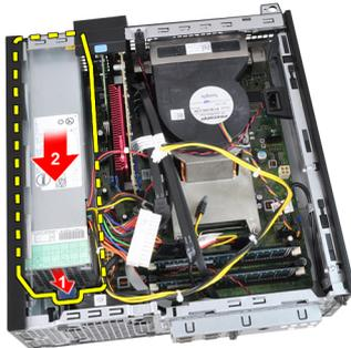
11. Lift the power supply out of the computer.
