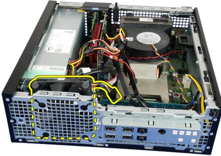
9. Pry up the grommets from the system fan and remove it.
