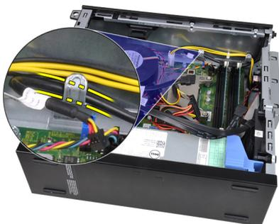
7. Pry the power-switch cable away from the chassis.
