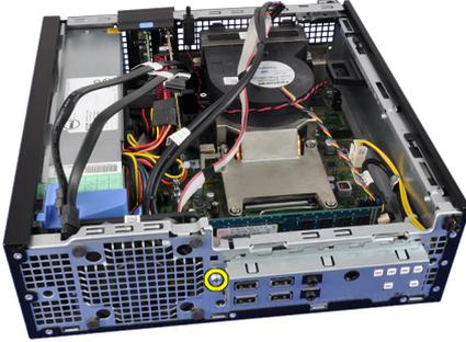
8. Slide the I/O panel towards the right of the computer to release it from the chassis.
