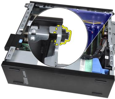
8. Slide the power-switch cable out through the front of the computer.
