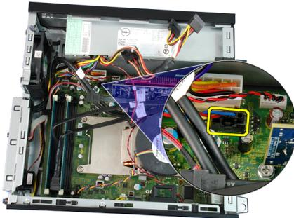
7. Slide the grommets inward along the groove and pass through the chassis.
