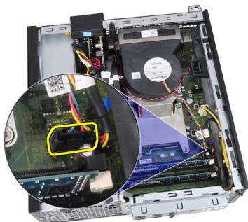
6. Release the Input/Output Board or the FlyWire cable from the routing channel on the heat sink.
