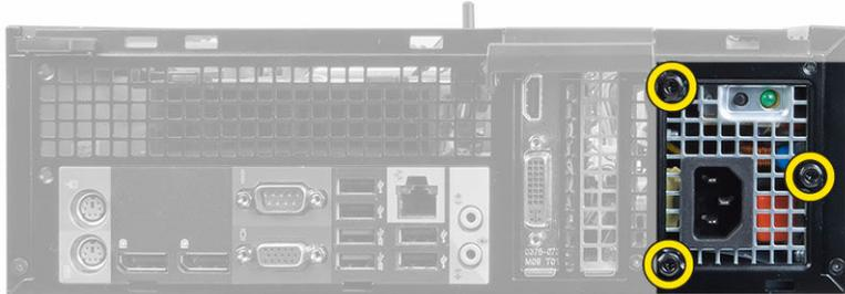
6. Push in on the blue release tab and slide the power supply towards the front of the computer.
