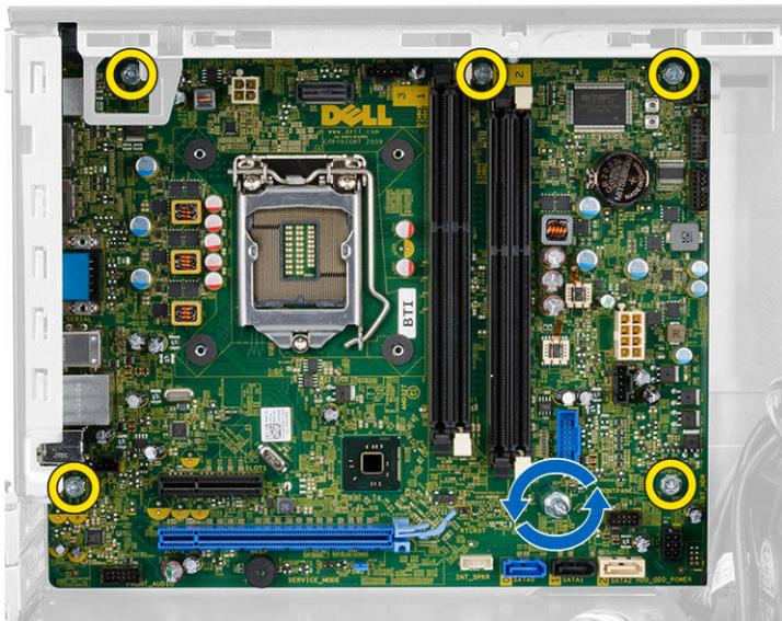
6. Remove the system board from the chassis.
