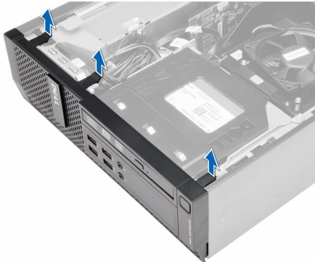
4. Rotate the bezel away from the computer to release the hooks on the opposite edge of the bezel from the chassis. Then, lift the chassis and remove the front bezel from the computer.
