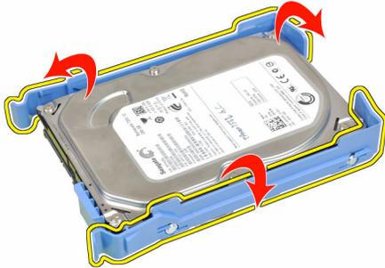
5. Remove the screws that secure the mini hard drive to the hard-drive bracket and remove the hard drive from its bracket.
