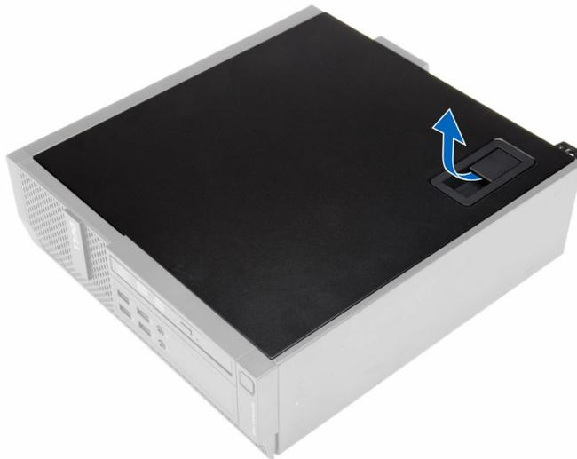
3. Lift the cover upward to a 45-degree angle and remove it from the computer.
